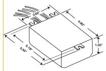
Center line to center line is .16" less than end to end on models with mounting feet.
